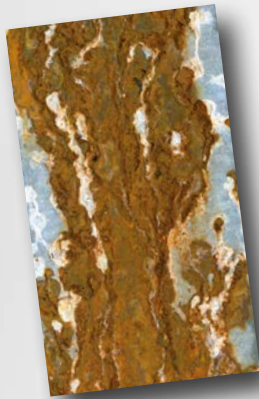
Hot dip galvanised 20 µm after 6 weeks
