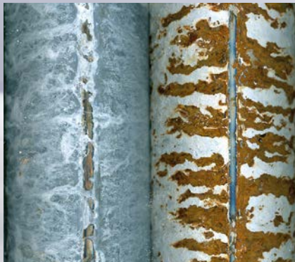
Magnelis® ZM120 welded, not re-protected
