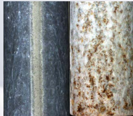
Magnelis® ZM310 welded and re-protected
